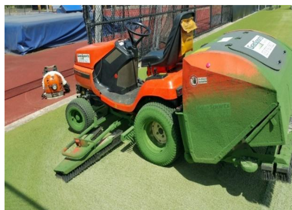
Photo 9: The yarn has been exposed to UV and the tips are breaking down and covering the maintenance machine
