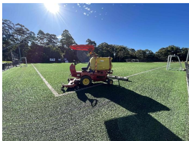
Photo 10: Machinery, including the metal magnet at rear (Source: Sports Clean)
