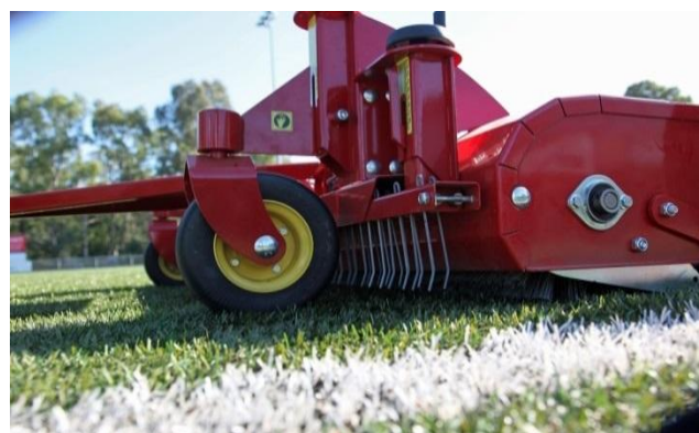
Photo 7: Modern machine providing height options for the tines to be used into the turf by an experienced operator
